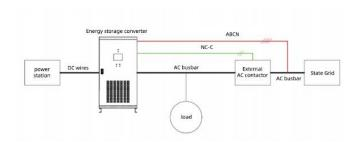
After a power outage in the grid, if the PCS needs to operate in grid-forming mode, a solution with one AC output port and an external AC contactor is required. The external AC contactor is an optional component. The energy storage converter will reserve dry contact terminals for external control of the AC contactor and terminals for AC voltage signal sampling. Users need to provide their own wiring (1mm²). The operating logic is as follows:
